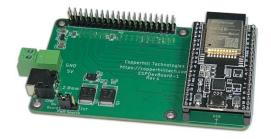
The *espBerry* DevBoard combines the <u>ESP32-DevKitC development board</u> with any Raspberry Pi HAT by connecting to the onboard RPicompatible 40-pin GPIO header.
