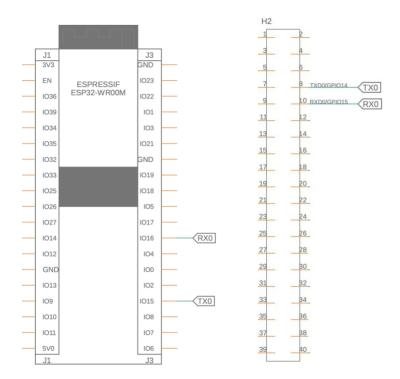
We have chosen not to use the standard RX/TX (GPIO3/GPIO1) signals on the ESP32 DevKit, since they are often used for test prints through the Serial Monitor of the Arduino IDE. This may interfere with the communication between the ESP32 and the RPi HAT. Instead, you must map IO16 as Rx and IO15 as Tx per software as explained in the *Software* section of this manual.
