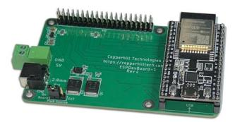
The *espBerry* DevBoard combines the <u>ESP32-DevKitC development</u> <u>board</u> with any Raspberry Pi HAT by connecting to the onboard RPi-compatible 40-pin GPIO header.
